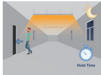
III. The sensor turns OFF light automatically after the holdtime.
