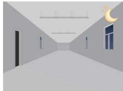
V . The sensor keeps light ON for holdtime period after motion leaves.
