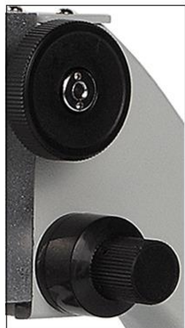
Separate Coarse and Fine Focusing Knobs, Coarse Focusing Range:50mm, Fine Adjustment Range :1.8mm- 2.2mm
