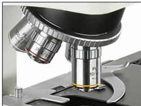
Infinity Plan Achromatic Objective 4x/0.1, 10x/0.25, 40x/0.65(S), 100x/1.25(O,S)
