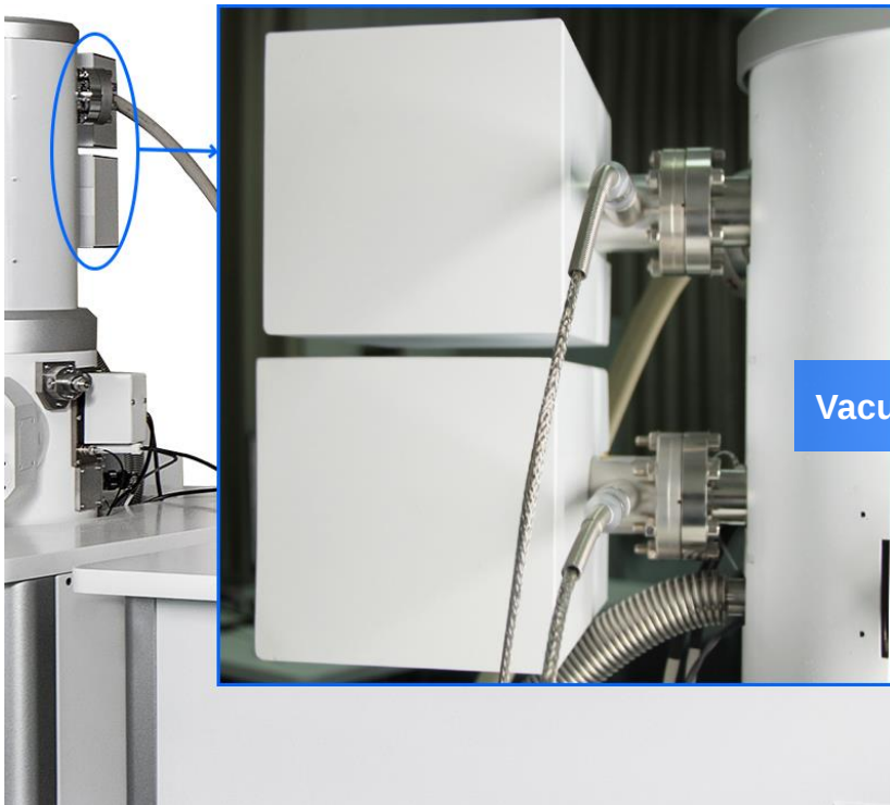
Schottky Field Emission Gun Electron Gun Electron Gun Room Vacuum >2 \times 10^{-7} Pa
