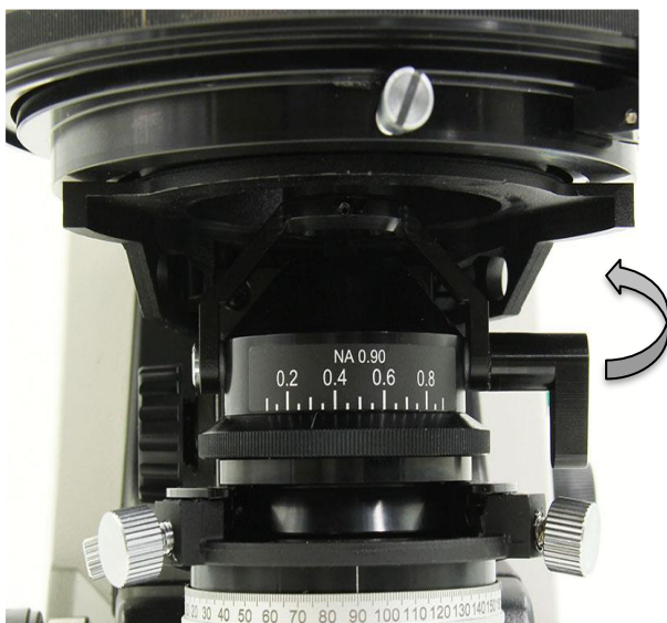
Swing-out NA0.9/0.25 Abbe Condenser with Iris Diaphragm & Filter
