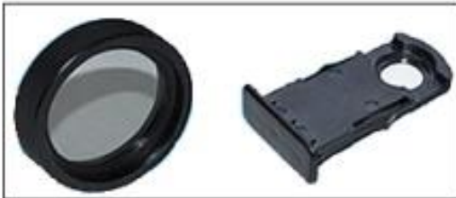
Simple Polarizing Attachment Optional Polarizer Used On Light Collector Of Base, Analyzer Inserted Into Hole on Nosepiece
