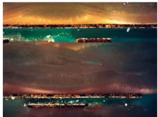
PCB Cross Section 20X Simple Polarizing
