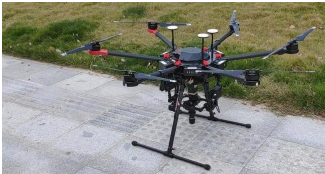
Figure 16 Drone-borne hyperspectral imaging camera
