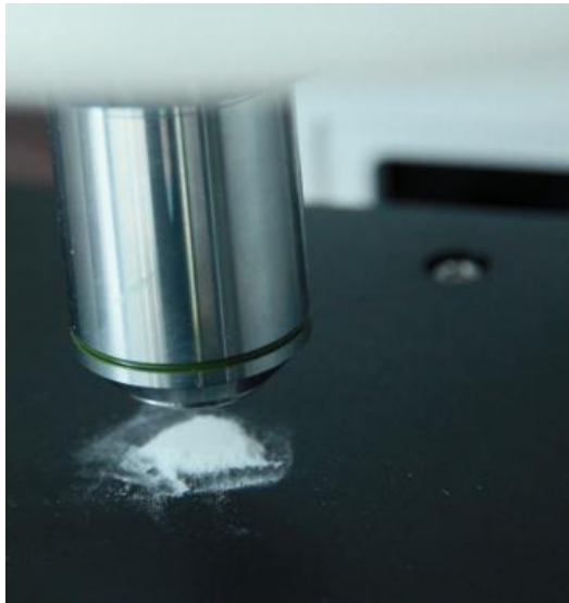
Figure 21 High transmittance objective for Raman signals. Objective focal length up to 8 mm.
