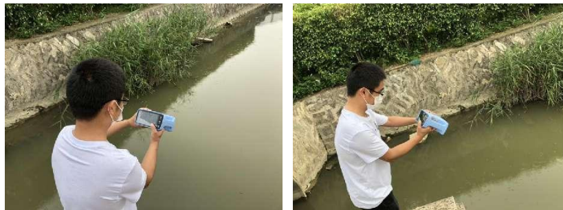
Fig 8 In April 2020, the Aositiancheng ATP9100 ground-based spectrometer monitored the red tide in Sandu Bay, Ningde, Fujian province
