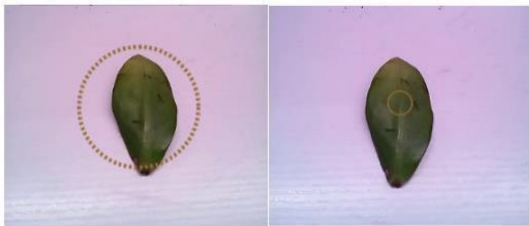
Fig 3 Comparison of measurement ranges between 25° field-of-view lens and 5° field-of-view lens
