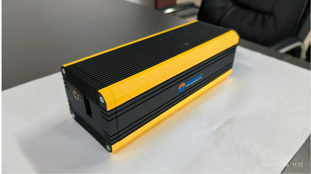
Figure 4 ATH1080K/ATH1080KW Hyperspectral Imager
