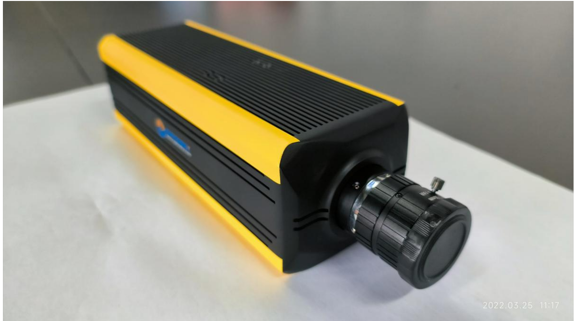
Figure 3 ATH1080K/ATH1080KW Hyperspectral Imagers (Core: ATH1080 and ATH1080W, respectively)
