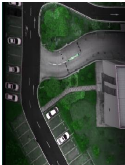
Figure 2. Hyperspectral Flight Data of ATH9010Z Series UAV (Flight Location: Institute of Rare Earth Materials, Chinese Academy of Sciences, Jimei District, Xiamen, Fujian Province; Flight Altitude: 100m; Airspeed: 6m/s; Wind Speed: Level 3)
