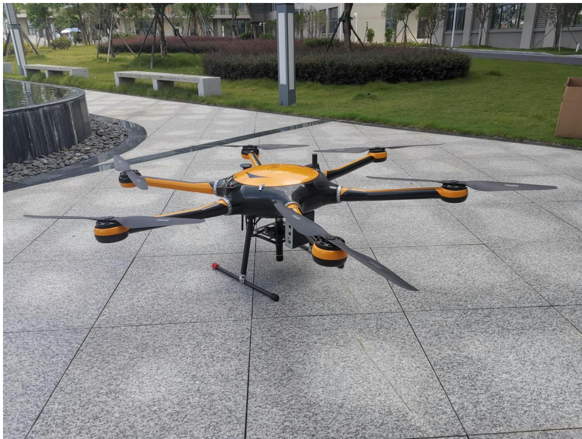
Fig 12 Drone hyperspectral imaging camera, developed and designed by Optosky
