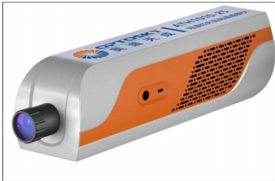
Fig.4.1 Physical image ofATH101R-25 hyperspectral imager
