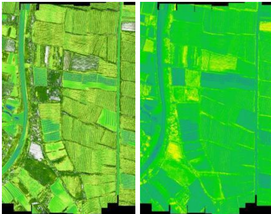
Figure 6.6 Vegetation Inversion Results from ATH9010 Hyperspectral Drone (Greener color = Healthier growth)
