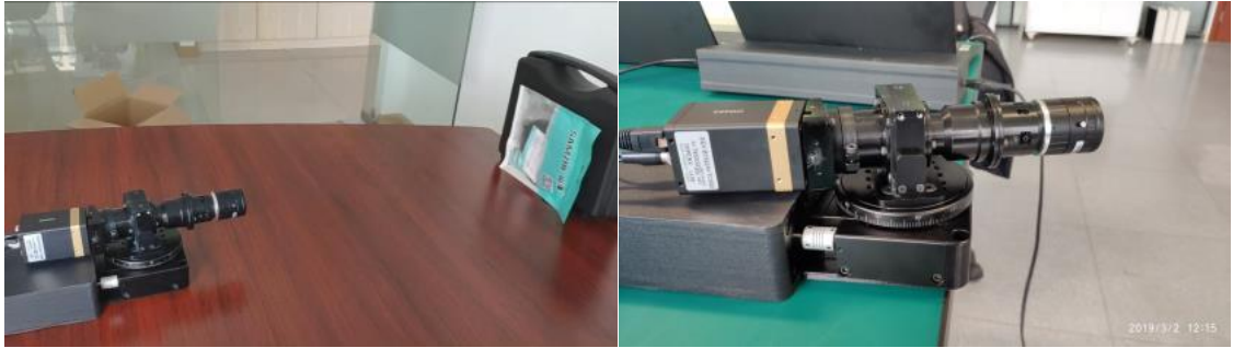
Fig. 1 Previous-generation rotary-scanning hyperspectral imager manufactured by Optosky
