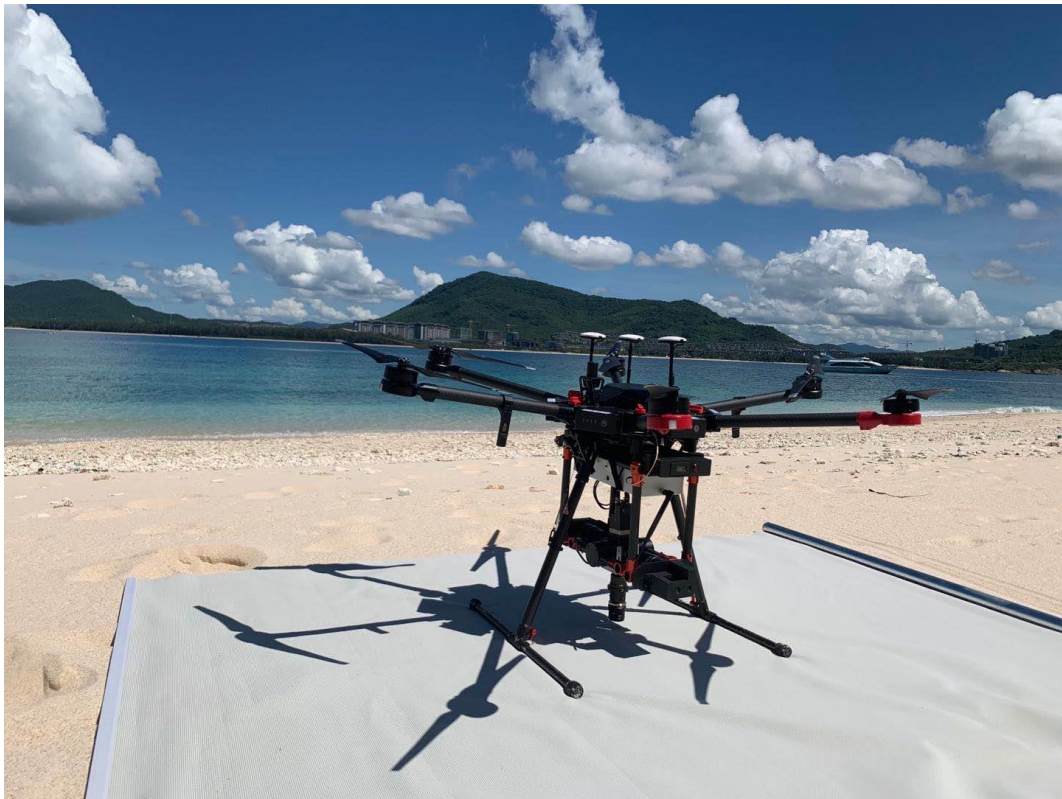
Figure 34: Optosky UAV hyperspectral imaging system
