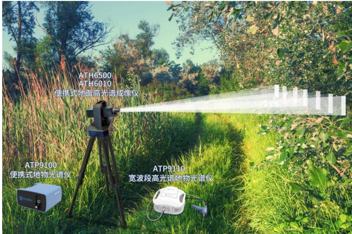
Figure 4 Combined application of hyperspectral imager and field spectroradiometer
