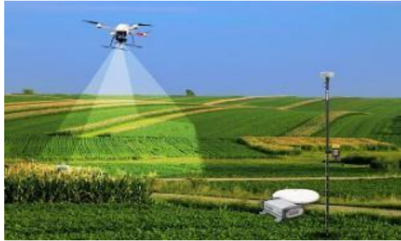
Figure 1 Schematic diagram of hyperspectral flight of ATH9100 UAV
