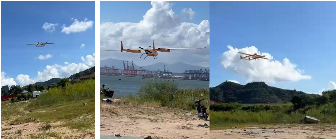
Figure 7 Flight scene of ATH9100-FW and ATH9100W-FW vertical take-off and landing fixed-wing UAVs equipped with hyperspectral imagers
