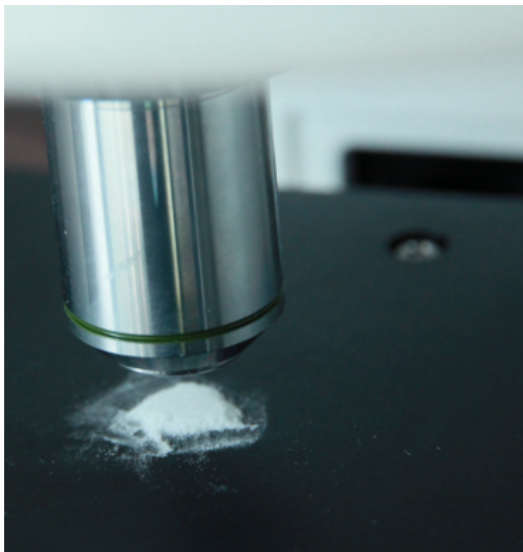
Fig 15 Raman signal high throughput objective, focal length reach up to 8 mm;
