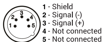
DMX-input XLR mounting-plugs (rear view):
