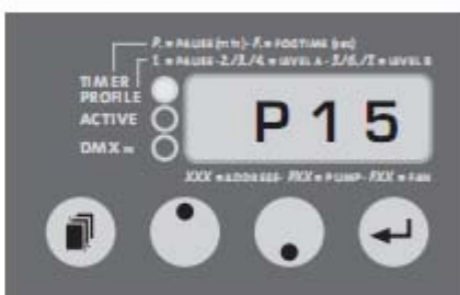
Fig. 13: Adjusting the pump
