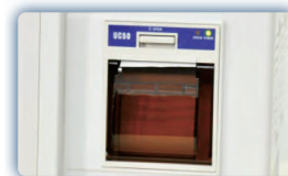
Supports the print of 3-channel waveform at the same time.
