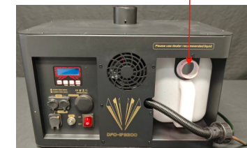
Smoke Oil Filling
