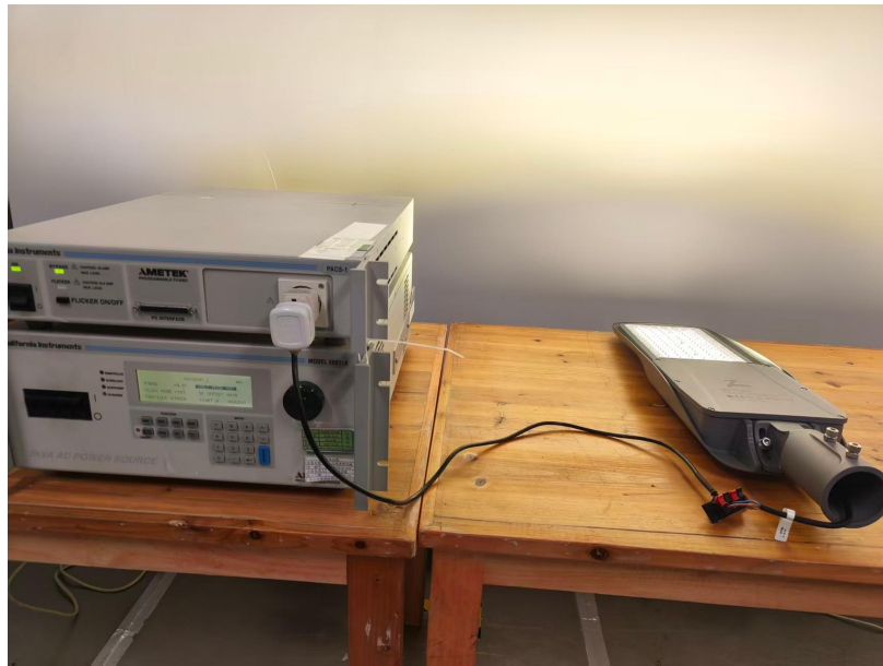
Photo 4 Harmonic & Flicker Test Setup
