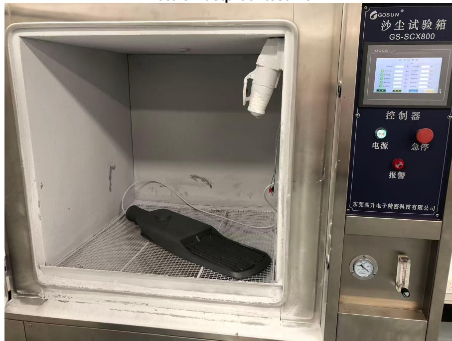
Photo 3 Dustproof test view
