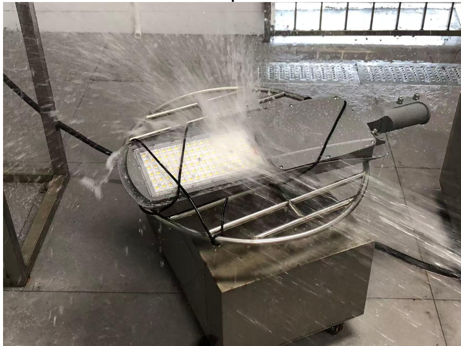
Photo 4 Waterproof test view
