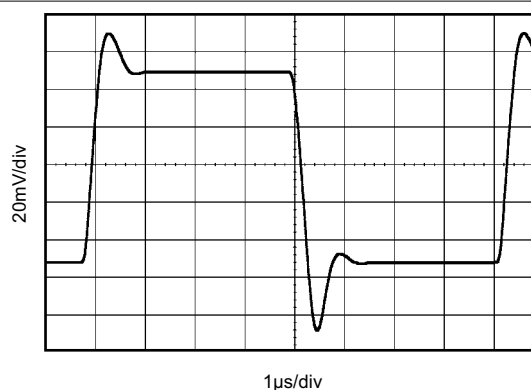
Figure 6-20. Large-Signal Step Response
