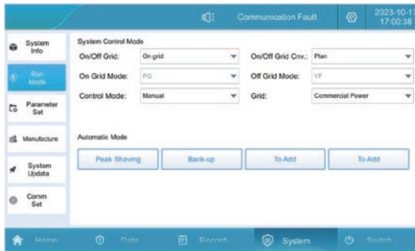
Figure 5.9 Grid-connected manual mode setting
