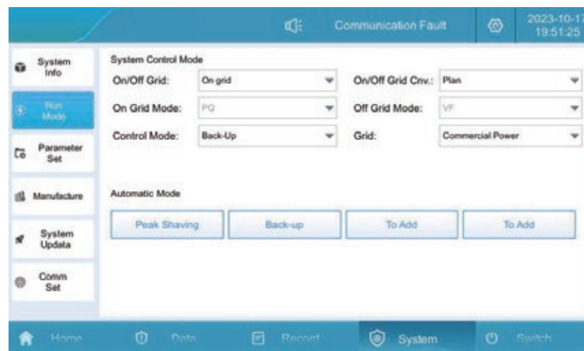
Figure 5.18 backup control mode
