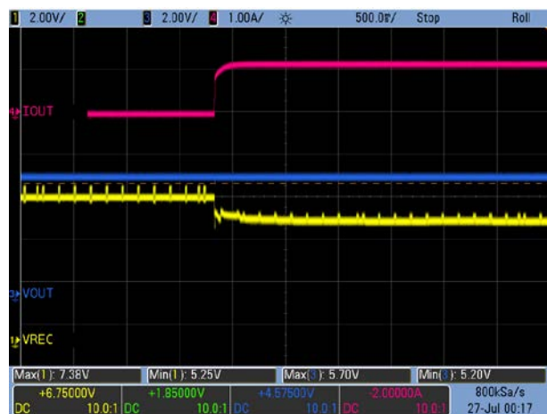
Figure 11. Load Transient: V_{OUT} = 5V , 0A \rightarrow 1.2A
