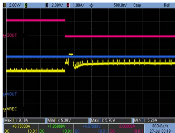
Figure 12. Load Transient: V_{OUT} = 5V , 1.2A \rightarrow 0A
